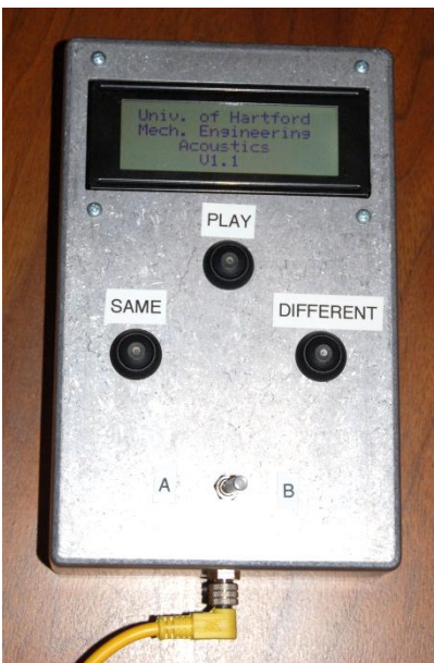
Figure 1: Custom subject-interface control that allows subjects to toggle between Signals A and B in real-time.
