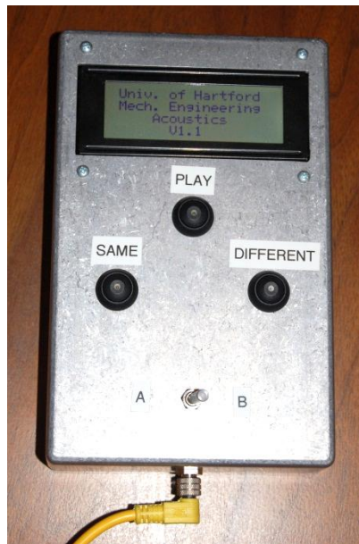
Figure 2: Custom subject-interface control that allows subjects to toggle between Signals A and B in real-time.
