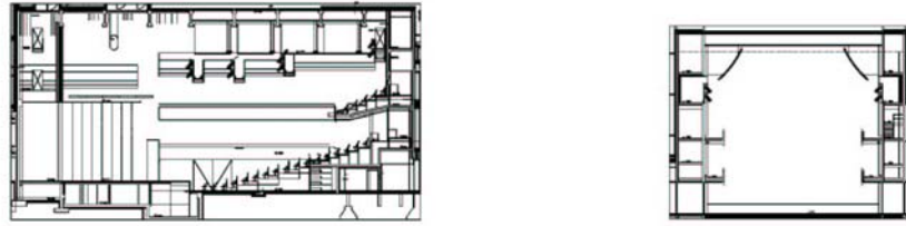
Figure 6 - Length and cross section of the Verkatehdas Hall
