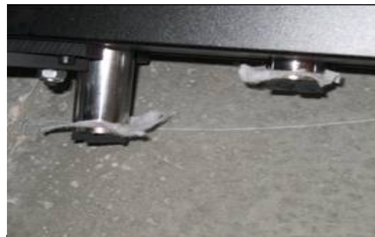
Figure 8: Magnets Attached to the Tapping Machine
