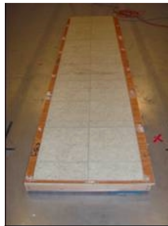
Figure 4: Profile 9, Thick Vinyl Sheet Covering on Sub-floor
