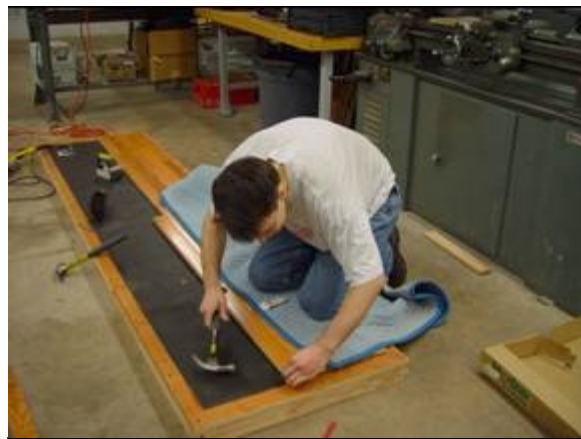
Figure 5: Construction of Profile 10, Oak Flooring
