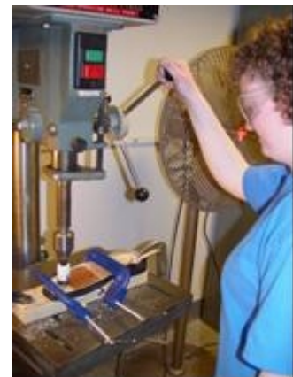
Figure 6: Coring the shoes for the tapper
