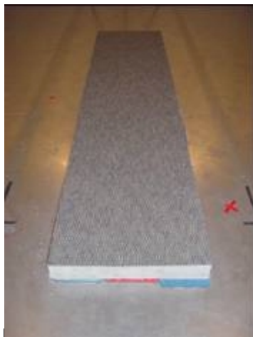
Figure 3: Profile 3, Rubber-Backed Carpet on Concrete
